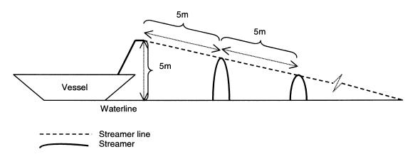
(i) The streamer line needs to protect baited hooks from seabirds. This means that the streamer line should be positioned in such a way that streamers are flapping in an unpredictable fashion, above the area in which the baited hooks enter the sea, so that seabirds are deterred from attempting to take bait from the hooks. In order to achieve this even during cross-winds, it is expected fishers will have to make adjustments to the configuration of the streamer line depending on the conditions.
